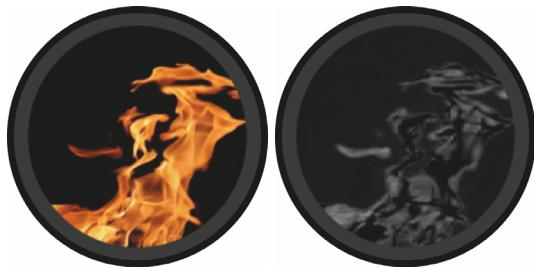
Only when an incident looks like fire visually *and* looks like fire in the infrared spectrum does the FCam signal an alarm condition. This allows the FCam to be extremely sensitive to fire and yet reject almost all false alarms.
